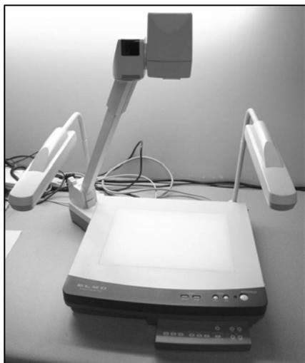
**Camera Head:** The camera head captures the image of the document which is then transmitted to the screen of the telemedicine system
