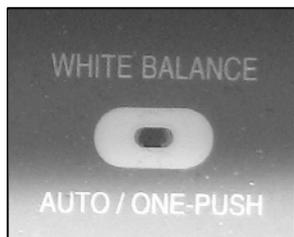
**Adjusting the White Balance:** The white balance refers to the correctness of color reproduction under various lighting conditions. To adjust the white balance of the camera:
