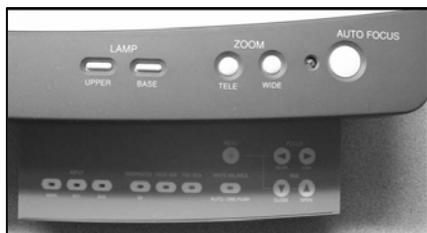
**Front Panel:** The front panel is a dashboard and controls the functionality of the Document Camera. The following are some of the buttons and associated indicator lights. Please note that different versions of the Document Camera will have slightly different setups.
