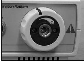
**Adjusting the Light Intensity:** The light intensity control knob is located around the outside of the light cable connector (the right side of the Light Box). The intensity ring controls the amount of light in the scope:
